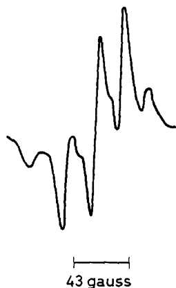
Figure 11—E.s.r. spectrum of crystalline methacrylic acid at 77°K after treatment with the discharge at 77°K
