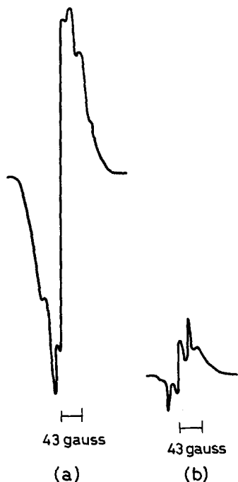
Figure 10—E.s.r. spectrum of polymethacrylic acid after treatment with the discharge at 77°K. (a) Immediately after treatment: (b) after 10 min at 20°C
