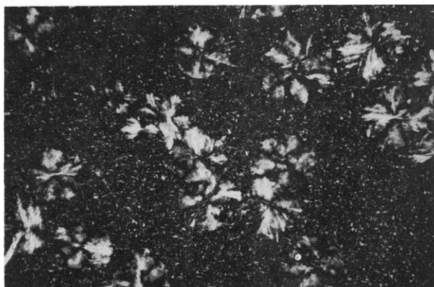
Figure 16—Fraction 2, crystallized at 130°C, between crossed nicols ( \times 62 )
