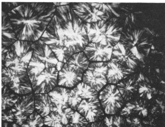
Figure 12—Total sample M, crystallized at 130°C, between crossed nicols ( \times 62 )
