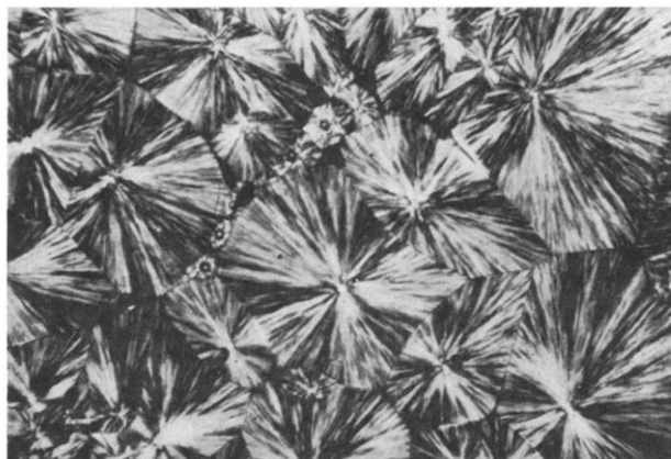
Figure 18 —Fraction 4, crystallized at 130°C; between crossed nicols ( \times 62 )
