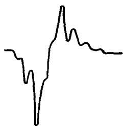
Figure 7 —E.s.r. spectrum of polypropylene powder after treatment with discharge at 20°C
