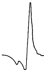
Figure 14—E.s.r. spectrum of polymethyl methacrylate at 77°K. The specimen was treated with the discharge at 77°K then warmed to -80°C in the presence of air for 1 min before recooling
