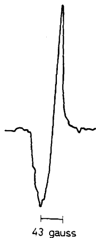
Figure 16—E.s.r. spectrum of peroxy-radicals from poly-vinyl chloride at 20°C produced by admitting air to the specimen of Figure 15 at 20°C
