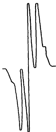
Figure 4 —E.s.r. spectrum of crystalline itaconic acid at 20°C after treatment by high-frequency discharge at room temperature
