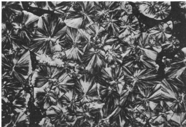
Figure 13—Ether residue A, crystallized at 130°C, between crossed nicols ( \times 62 )
