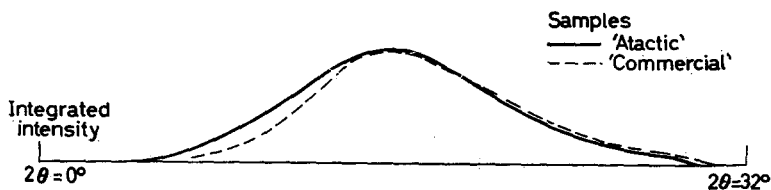
Figure 1 —Traces of two samples of polypropylene in the melt from high temperature X-ray photography
