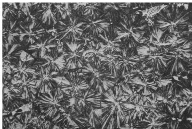
Figure 19 —Fraction 5, crystallized at 130°C, between crossed nicols ( \times 62 )
