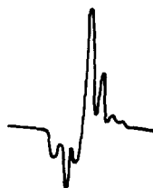
Figure 13—E.s.r. spectrum from polymethacrylic acid at 77°K. The specimen was treated with the discharge at 77°K, then warmed to 18°C in the presence of air and held at that temperature for 3 min before recooling to 77°K
