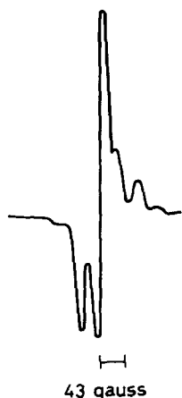
Figure 2 —E.s.r. spectrum of peroxy-radical from polyethylene at 77°K produced by admitting to the specimen of Figure 1 at -80°C
